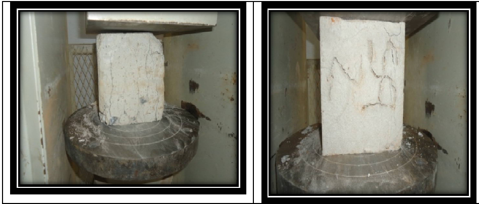
Figure 6: Cubes testing for compressive strength (2% fibre)
