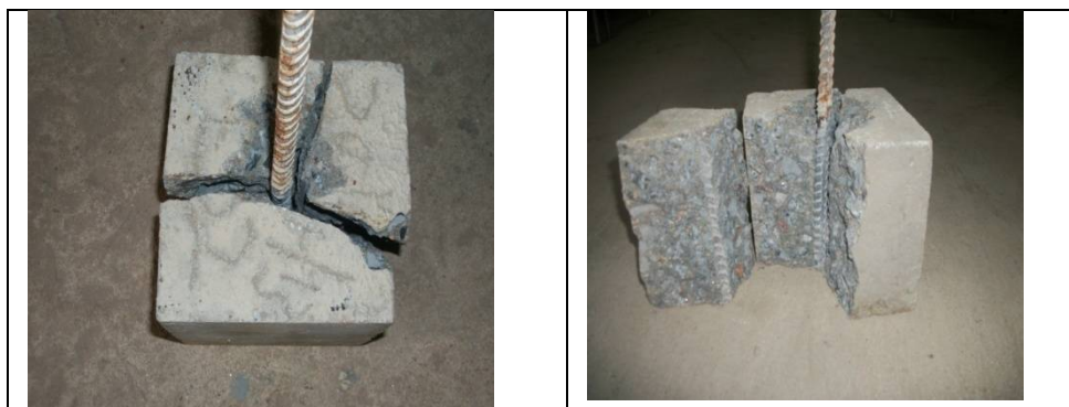
Figure 7: Failure mode of cube using 0% fibre (Pullout)
