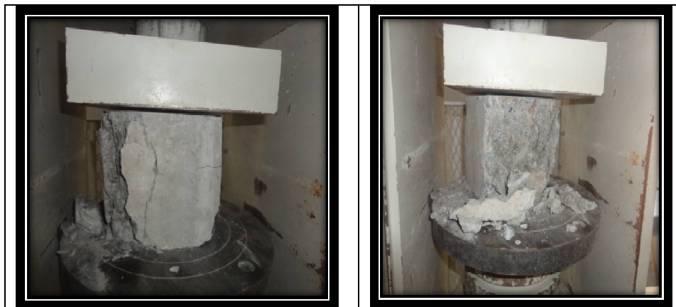
Figure 4: Cubes testing for compressive strength (0% fibre)
